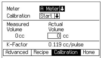
Fig. 68. Calibration Screen
